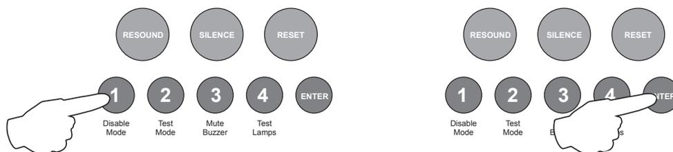
When finished, press and hold Button 1 (Disable Mode) for 3 seconds or alternatively wait approx 10 seconds and the panel will save the settings and revert back to Level 3 access mode.
