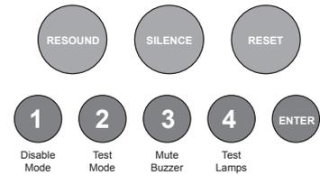
To access Level 3 options, first set switch 3 on the 3 way DIL switch located on the main PCB to the 'ON' position. Then activate the controls by turning the key switch or by entering the four digit code (see Activate Controls in the OPERATING section).
