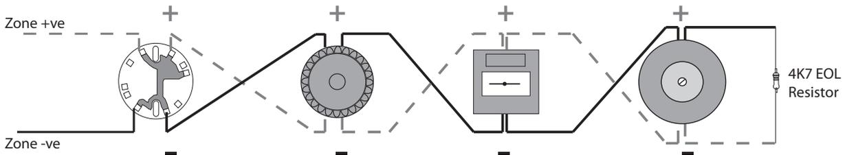
Haes Twin Wire systems require special 'sav-wire' detector bases and polarised call points but standard sounders. Most modern, non addressable, low current, polarised sounders, bells and beacons are compatible, Cooper Fulleon, Besson, Klaxon etc.
