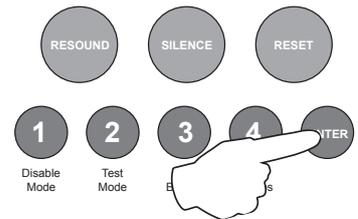
When all disablements have been set, press and hold the Disable Mode button for 3 seconds again. This will exit the disable selection mode and the panel will return to standby. All disabled circuits and the General Disablement will now be indicated by a steady LED.
