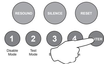
When finished all the zone function programming, enter the next programming code or disable the controls and return DIL switch 3 to 'OFF'.
