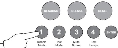
The setting of the attribute is indicated by the amber, fault / disabled / test LED, ON or OFF.
