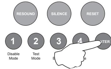
When at the sounder status position, use the ENTER button to toggle between testing with or without sounders. A rapid pulse = with sounders (default), a slow pulse = without sounders.
