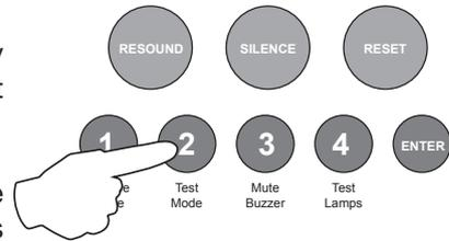
After 3 seconds the panel will bleep and the Test Mode LED and Zone 1 Fault/Disabled/Test LED will pulse slowly, indicating that Zone 1 is in test selection mode. The Sounder Status LED will also be pulsing rapidly, this indicates that the test will be **with** sounders. (Test mode without sounders is explained below)
