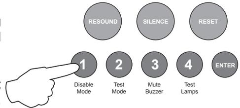
Pressing the Disable Mode button again will move disable selection mode to Zone 2 and the Zone 2 Fault/Disabled/Test LED will be pulsing instead. Subsequent presses will move the selection to Zones 3 and 4.
