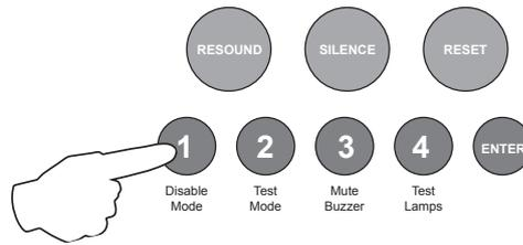
Press the ENTER button to return back to the zone selection, indicated by a steady zone fire LED
