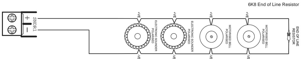
The sounder outputs can be configured to turn on continuously or to pulse (1s ON / 1s OFF).
