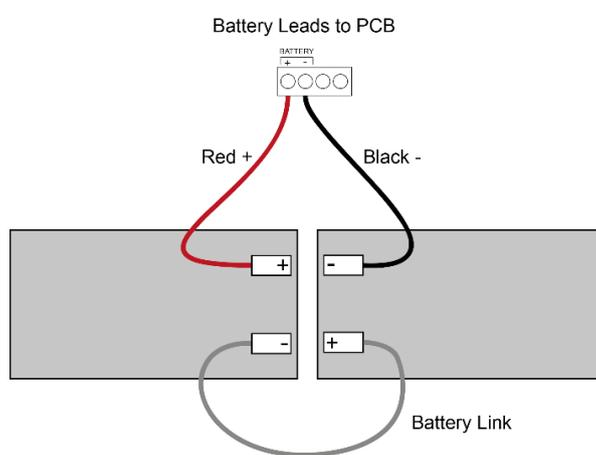
**Note:** In the event of mains failure, the battery charger circuit will protect the batteries from full discharge by disconnecting them when they reach below 19v. When the mains supply is restored the batteries will be automatically reconnected.
