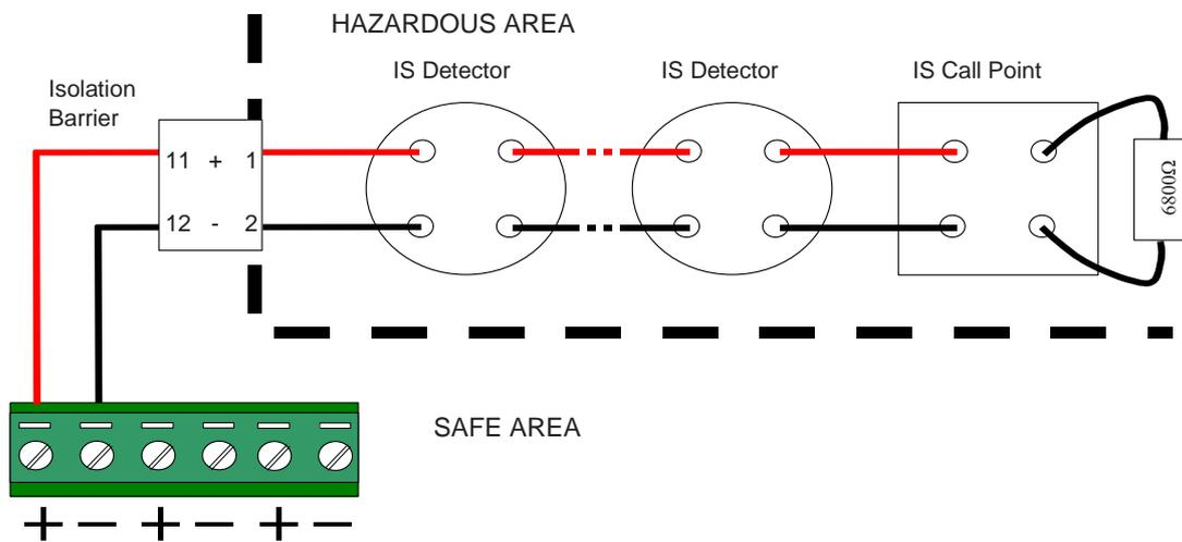
The recommended isolation barrier is an MTL Model: 5561 Only use intrinsic safe detectors and call points.
