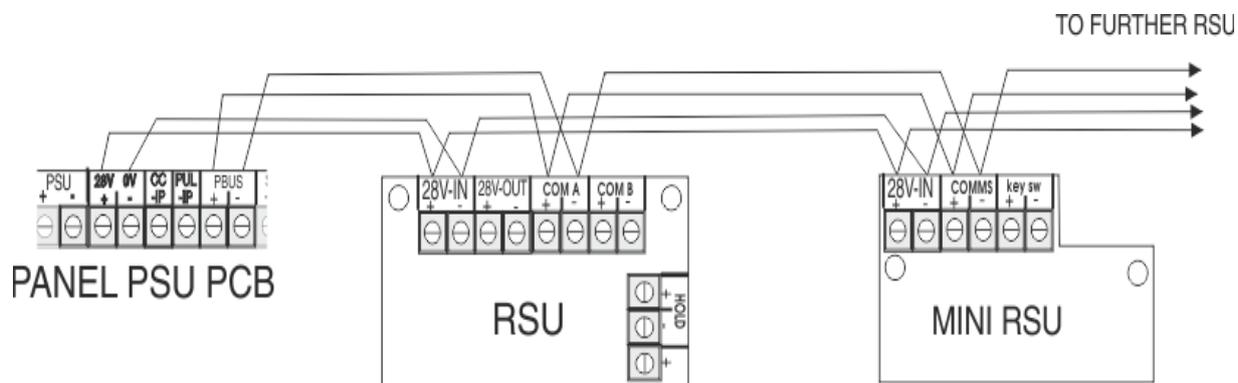
Each RSU has a PCB-mounted DIL switch and must be allocated a unique address between 1 and 16. When Two Flood zones are in use, it is possible to assign RSUs to either Flood Zone.
