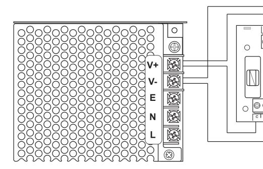
General wiring schematic showing connections to magnetic door retainers. TRX unit
