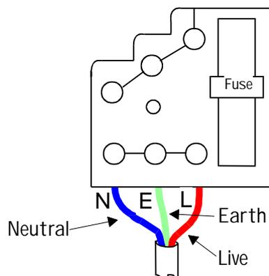
Figure 2 - Mains connection detail
