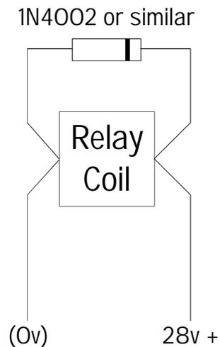
Figure 3 - Aux. relay connection detail
