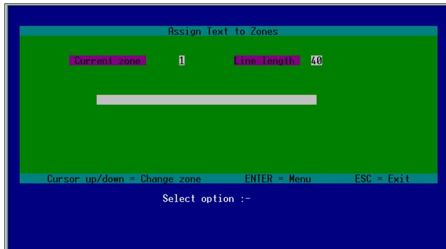
Select a zone in the range 1 to 84 via the up/down arrow keys and type in the appropriate zone text using either upper or lower case characters.
