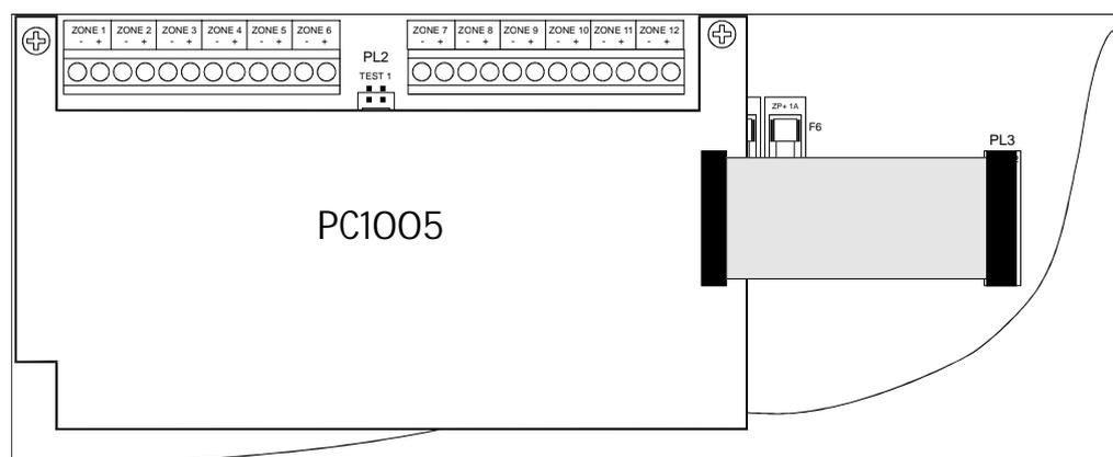
Figure 4 - PC1005 Mounting detail
