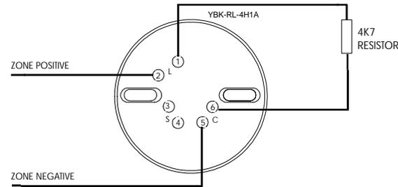
Hochiki "Safeline" Base YBK-RL-4H1A Should Be Used To Achieve Head Removal Monitoring With Haes 2000 & LEVEL Series Control Panels.
