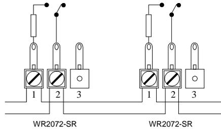
Standard Break Glass Call Point Connection Details With 470 OHM Resistor Fitted.
