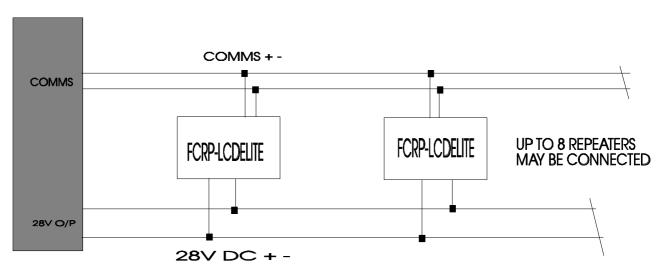
RECOMMENDED CABLE TYPE. SCREENED 2 OR 4 CORE. FIRETUFF, MICC, BELDEN OR SIMILAR .UNSCREENED CABLE NOT RECOMMENDED MAX LENGTH 2000 METRES.
