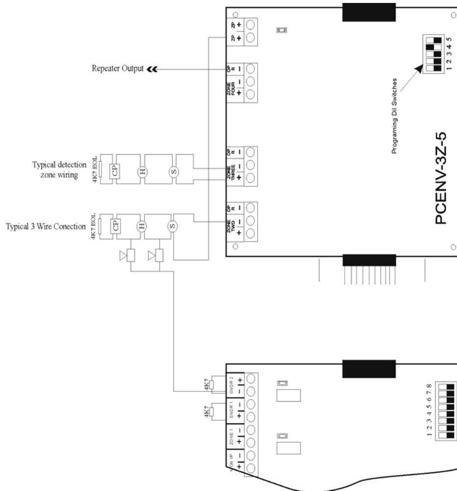
A typical 3 wire circuit is shown on Dwg No. S1599, connected into zone 2. This method of wiring does not meet current standards for new systems, but may be suitable for upgrading certain existing installations.
