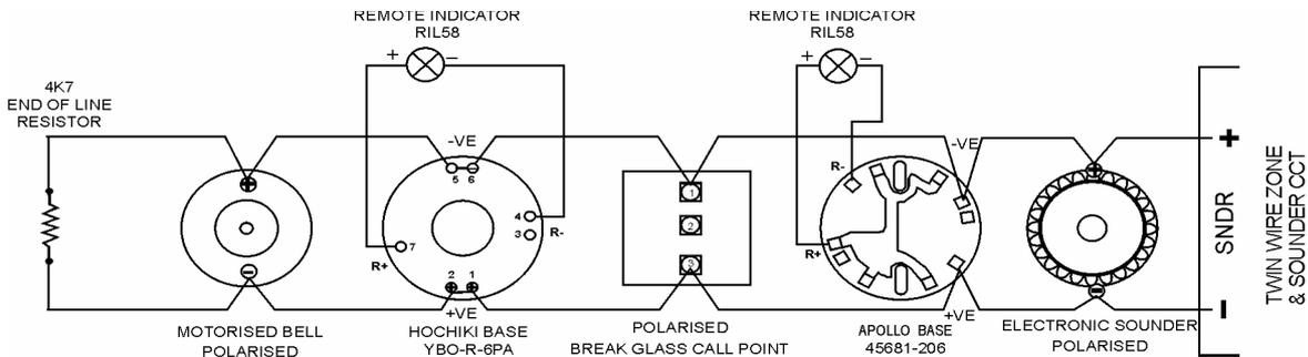
**Drawing shows TWIN-WIRE zone and sounder CCT connections when panel is in it's quiescent state (not in alarm). +ve wire goes to sounder +ve but to detector or call point -ve and vice versa.**
