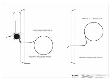
bar and fit a new roll of paper, ensure the loose end of the paper roll is facing towards the back of the lid . Feed the paper through the slot with the coated side uppermost. Re-fix the paper roll holder bar. Insert the lead of the paper roll up and under the rubber guide roller so that the coated side is against the lid, using the thumbwheel to advance the paper. The paper should appear from above the roller with the coated side uppermost.
