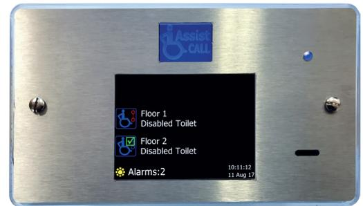
The HC-ACR connects to the Haesomm network via the nearest HC-EX8-8 system expander panel via Cat 5 cable, plugging in to a dedicated port. It can be located up to 30m away and does not require a power supply and does not take a line output.
