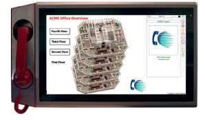
The HC-Commander is a replica of the master station (which still must be fitted) and allows hi-resolution maps or graphical representations to be displayed with buttons overlaid representing the EVCS outstations. Area buttons allow screens to be linked enabling overview and zoom screens to be quickly implemented.
