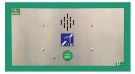
The HC-ILB has been designed to meet the requirements for a Type B outstation with an integral audio frequency induction loop (AFILS), the design has been optimised to produce the horizontal field as required by BS5839pt9:2011, overcoming the limitations traditionally associated with a wall mounted induction loop.
