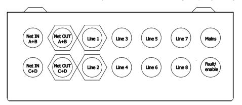
Unused knockouts must be left unopened to comply with the Low Voltage Directive. Accidentally knocked out holes should be blanked off.
