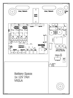
Prior to mounting the EX8, it should be decided if the field wiring is to be run on the surface or concealed. There are 14 knockouts on the top and 2 slotted entries with a dedicated mains supply entry at the rear. If a knockout is removed by mistake, fill the hole with a good quality cable gland.
