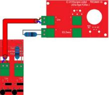
**Note:** The Earth screen should be sleeved and connected to the terminal block in the controller, and the earth stud in the Type A outstation.
