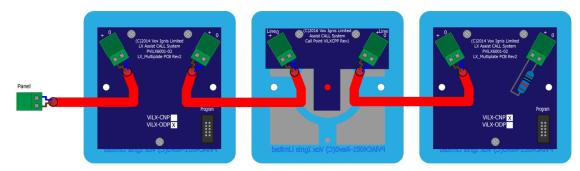
The "Assist Call" ACA kit comprises an Over door Indicator, a Pull Cord, and a Cancel Plate. The above order is a typical order; with the Over door Indicator, Pull Cord and the Cancel Plate connected as shown, but the plates can be wired in any order as long as the EOL resistor goes into the free terminal of the last plate.
