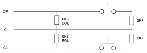
Each local vent control switch operates any number of vents depending on configuration. If the 2K7 resistor is replaced with a 10K resistor, the vent will open or close to a pre-configurable position. This operation can be used as a thermostatic control of the vent.
