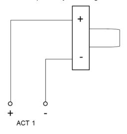
If an actuator output is not being used, a 6K8 resistor should be connected across the terminals. Alternatively, the circuit can be disabled from the config circuits menu.
