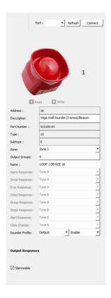
The Read and Write controls are used to transfer configuration data to or from the fire control panel, for the individual device.
