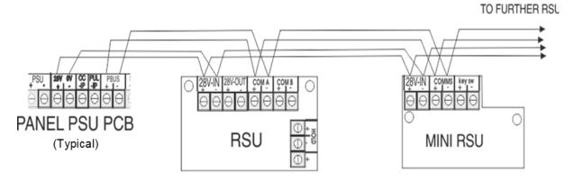
Each RSU has a PCB-mounted DIL switch and must be allocated a unique address between 1 and 16.
