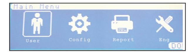
On the LCD screen, the box surrounding the menu icon is the cursor; this can be navigated through the menu options by using the Left/Right arrow keys to select required menu option and then pressing the  $\checkmark$  key.
