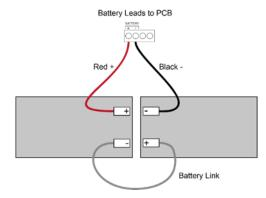
**Note:** In the event of mains power failure, the battery charger circuit will protect the batteries from full discharge by disconnecting them when they reach below 19v. When the mains supply is restored, the batteries will be automatically reconnected.
