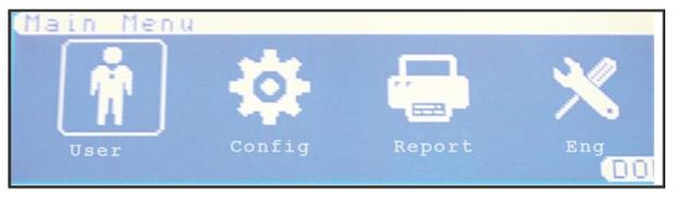
On the LCD screen, the box surrounding the menu icon is the cursor; this can be navigated through the menu options by using the Left/Right arrow keys to select required menu option and then pressing the  $\checkmark$  key.
