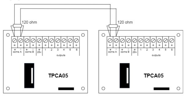
Each Network Card has a PCB-mounted DIL switch and must be allocated a unique address between 0 and 7 for panels and 8 and 15 for repeaters.
