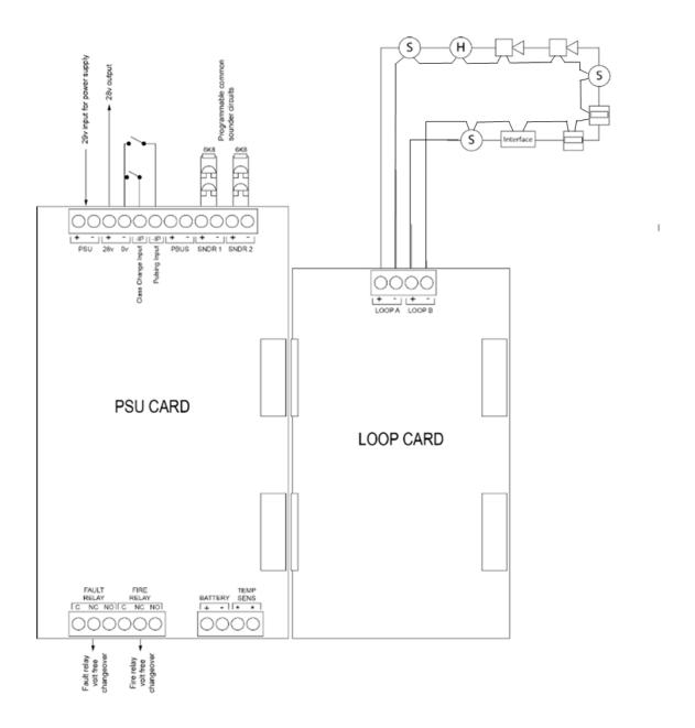
**Important note:** The first and last devices on the loop (those closest to the loop card terminals) must contain an isolator circuit. If these devices do not contain an isolator, dedicated isolators must be added at both ends of the loop.
