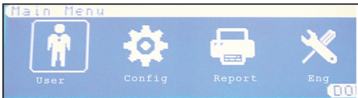
On the LCD screen, the box surrounding the menu icon is the cursor; this can be navigated through the menu options by using the Left/Right arrow keys to select required menu option and then pressing the ✓ key.
