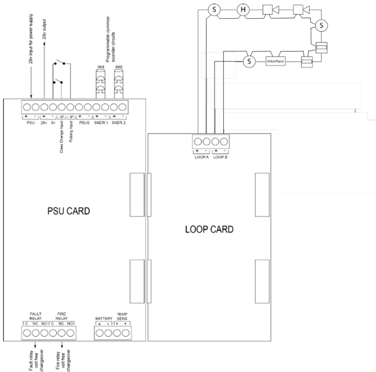
**Important note:** The first and last devices on the loop (those closest to the loop card terminals) must contain an isolator circuit. If these devices do not contain an isolator, dedicated isolators must be added at both ends of the loop.
