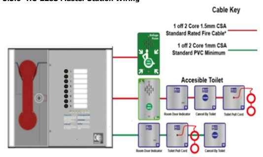
The wiring for a HC-228S Master Station is shown in the schematic below.
