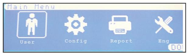
On the LCD screen, the box surrounding the menu icon is the cursor; this can be navigated through the menu options by using the Left/Right arrow keys to select required menu option and then pressing the  $\checkmark$  key.
