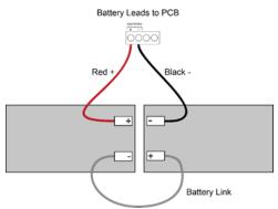
**Note:** In the event of mains failure, the battery charger circuit will protect the batteries from full discharge by disconnecting them when they reach below 19v. When the mains supply is restored the batteries will be automatically reconnected.
